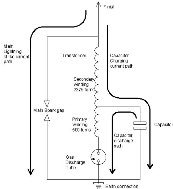
The diagram shows the capacitor charging path which is from the high voltage area of the finial and through the secondary of the transformer then through the capacitor and eventually to earth.
