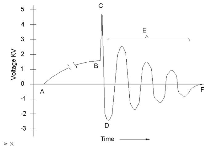
A – Start of capacitor charging (time A to B is unknown and depends on electrostatic charge)
